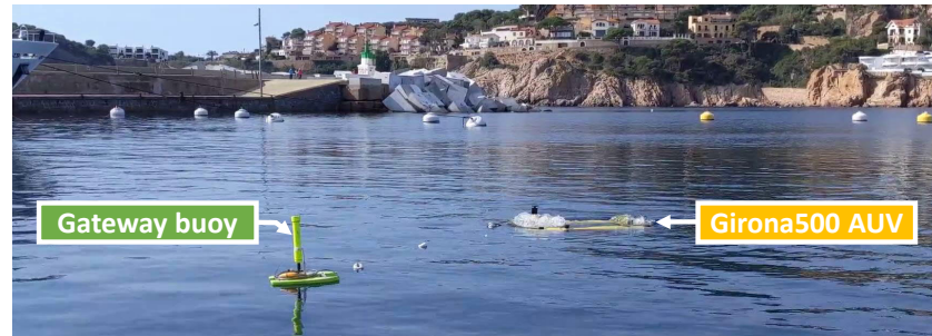
Figure 13. Girona500 AUV during the implementation of the path following algorithm at the harbor of Sant Feliu de Guíxols (Girona, Spain).
