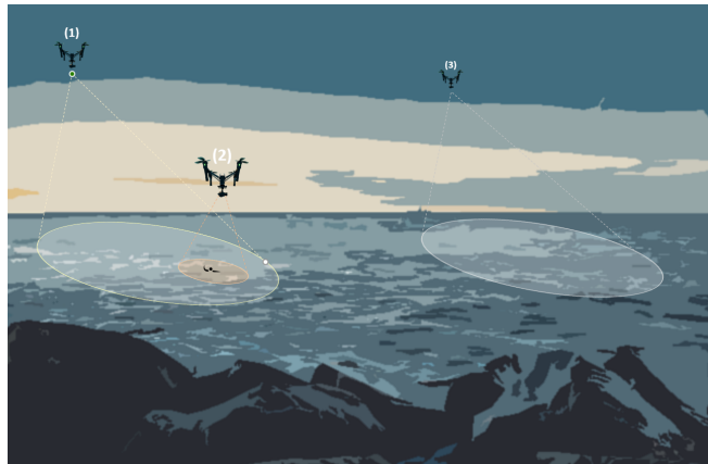
Fig. 1: Illustration of active-vision-based search in maritime environments with UAVs. A single UAV can first fly higher to cover larger areas and descend in the event of a positive detection to increase reliability. Search time can then be optimized by dynamically adjusting the altitude depending on the perception confidence.
