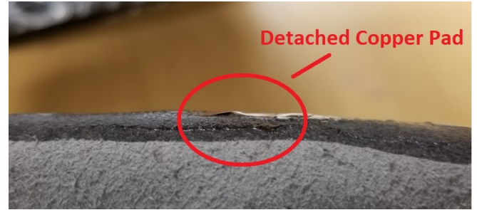
Fig. 7. Copper pads of RFID ICs detached from electro-textile antennas during washing: Inside thermoplastic elastomer platform (top) and inside encapsulant platform (bottom).
