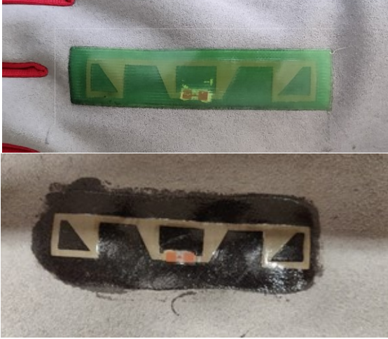
Fig. 2. Readymade glove-tag inside thermoplastic polyurethane (top) and stretchable encapsulant (bottom).
