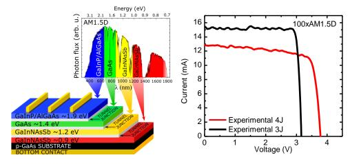
**Figure 1.** Schematic illustration of the processed four-junction solar cell structure (left). I–V characteristics of 3J and 4J cells fabricated on GaAs by MBE (right). The 3J cell is fabricated without the 3<sup>rd</sup> junction of the 4J design. The I–V curves were measured at continuous 100 suns illumination.
