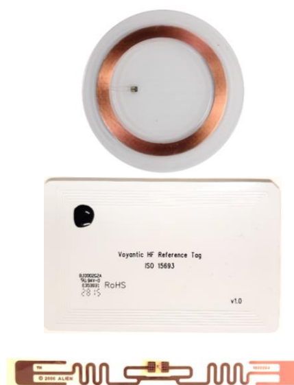
Figure 2: Commercially available RFID tags, LF (Top), HF (Middle) and UHF (Bottom).
