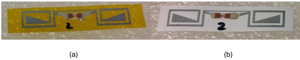
Figure 32: Thermal printed Tag design 1 on: (a) Kapton (Al) (b) THERMLfilm (Al).
