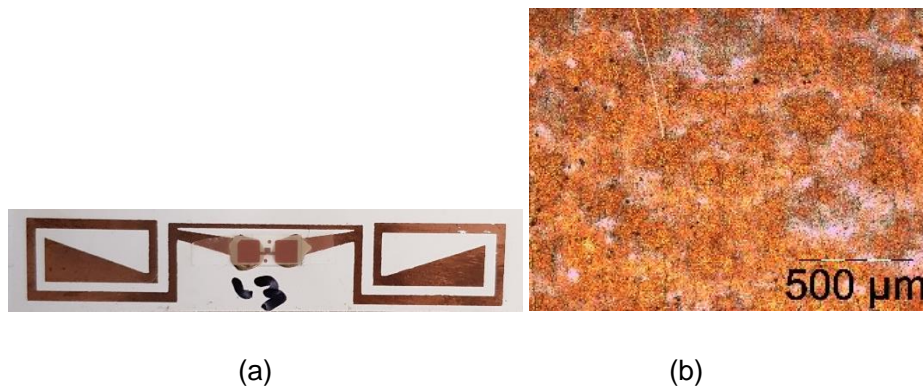
Figure 42: Ready tag: (a) Thermal printed Cu tag (b) Microscopic picture of the surface. [Publication III].
