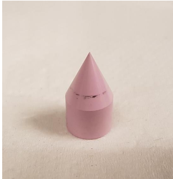
Figure 12: Typical nozzle of Nscript 3D dispensing system.
