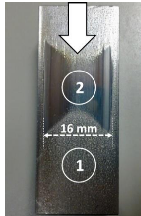
Figure 5: A typical wear track on an unrelated AISI 316L sample. Water feed and sliding direction is stated with an arrow and roughness measurement spots indicated by circles, pertaining to the numbering used in Table 5.
