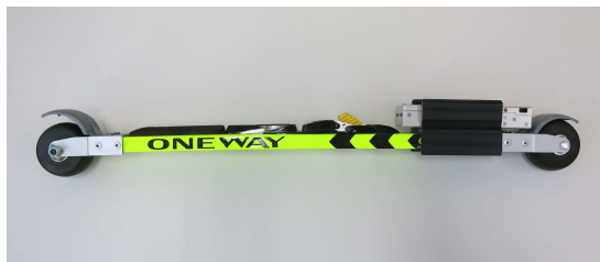
(b) The roller ski with the IMU in front of the binding.
