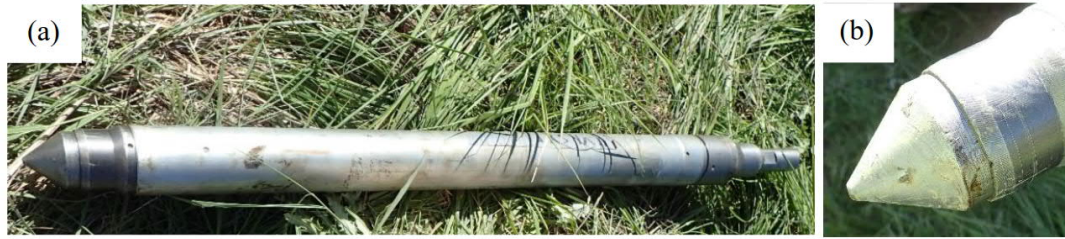
Fig. 7: ST:1 sampler with 50 mm liner; a) sampler apparatus before punching, c) detail of sampler used in Perniö and Lempäälä sites.
