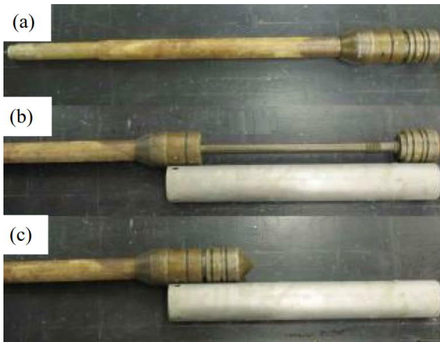
Fig. 8: Aalto 86 mm sampler, a) Aalto University version, b) sampling cylinder and outdrawn piston position, c) sampling cylinder and withdrawn piston position (Mataic, 2016).
