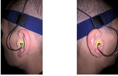
Fig. 1: Binaural microphone set worn by a test subject.
