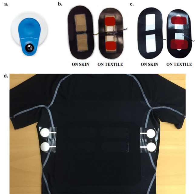
Fig. 2 a. Reference electrode, b. Textile electrode, c. Printed electrode, and d. Printed electrodes and interconnections integrated on the textile
