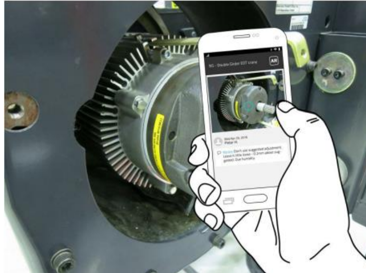
Figure 1. Concept image: accessing contextual social media in a maintenance task by means of object detection and Augmented Reality.
