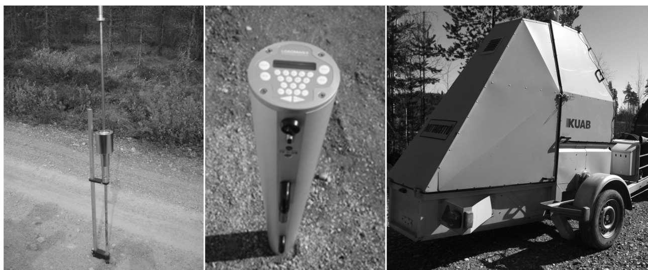
Fig. 2 Measuring devices: dynamic cone penetrometer, light falling weight deflectometer and falling weight deflectometer
