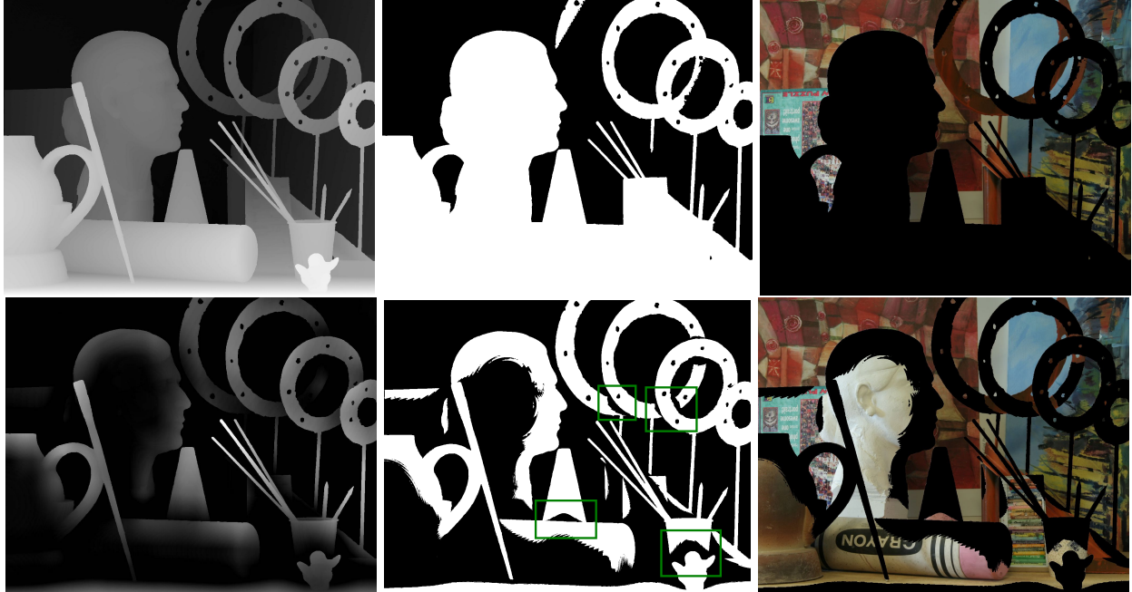
Figure 2. Foreground segmentation by locally-adaptive thresholding for the Art dataset. First row: Given disparity map D(\cdot) , foreground mask obtained by absolute thresholding as in, 12 corresponding background layer image; second row: positive part of the residual image ( D - D_{avg} ), foreground mask obtained by locally-adaptive thresholding, corresponding background layer image
