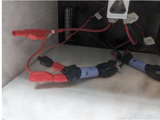
(b) NMC-based Li-ion battery cell placed in the climatic chamber.
