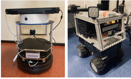
Fig. 3: The robots: A Turtlebot2 (left) and a Robotnik Summit XL Steel (right)
