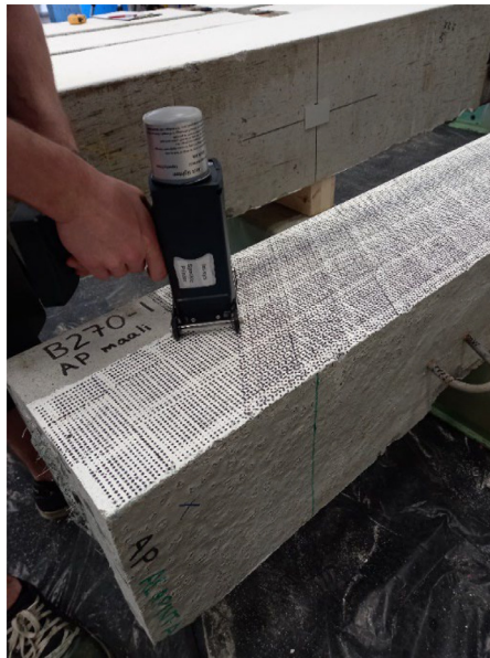
Fig. 8. Applying a black spackle pattern to the white-colored surface of the concrete piles.
