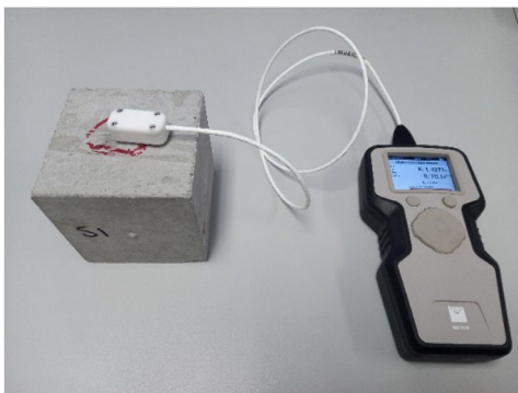
Fig. 2. Thermal property measurement using TEMPOS device.
