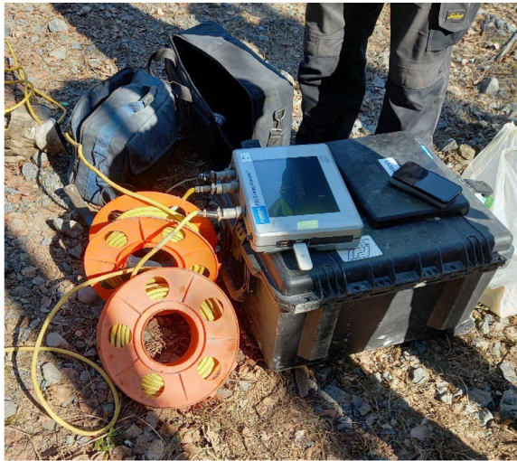
Fig. 3. PDA device for stress monitoring.
