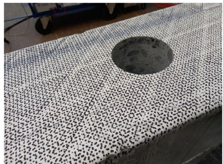
Fig. 1. Photos of some of the core specimens taken from the energy piles after flexural tests.
