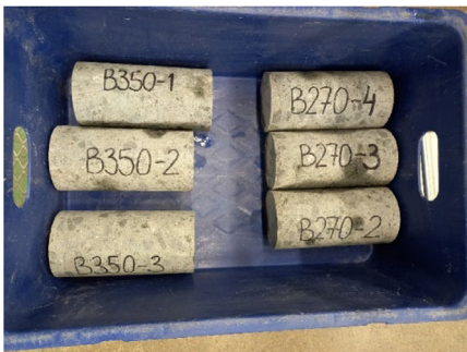
Fig. 1. Photos of some of the core specimens taken from the energy piles after flexural tests.
