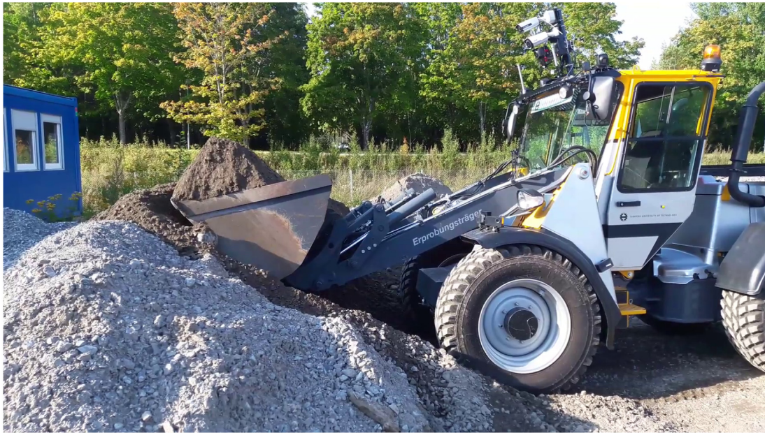
Fig. 7. An example autonomous HDMM (wheel loader) that was built at Tampere University with the cooperation of industry.
