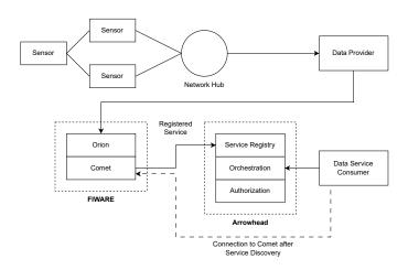
Fig. 3. System architecture for the implementation.
