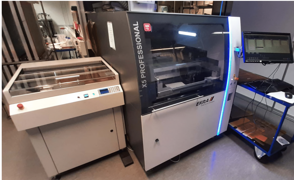
Figure 4.2. Screen printing system of Ekra X5 professional stencil printer.
