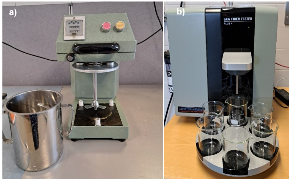
Figure 16. a) L&W wet disintegrator and b) L&W Fiber Tester device.
