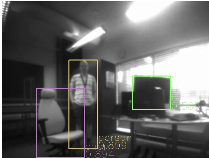
Figure 4.9. An image captured by AI-deck with added AI object detection results.
