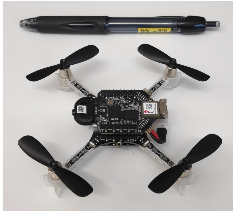
Figure 4.2. Crazyflie 2.1 with an AI-deck expansion deck on top. Also a pencil for scale.
