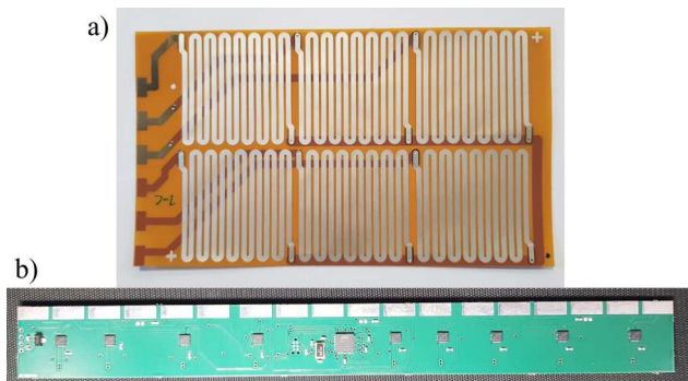
Fig. 4. a) A screen-printed flexible heating element (on the top) with the etched current distribution lines (on the bottom), b) heating electronics for the heating elements, where the microcontroller, nine load switches and rectangular contact pads are visible.
