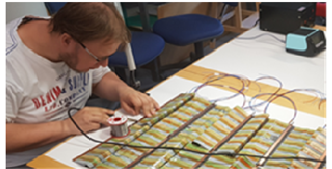
Fig. 3. Assembly of the display with three-colored pixels and carbon fiber heating elements.
