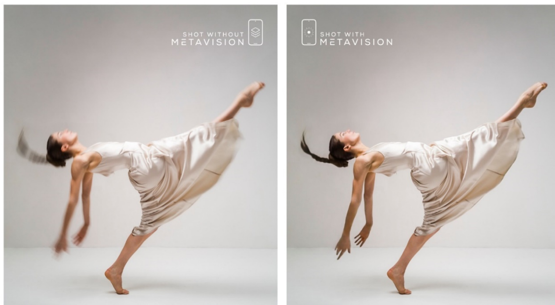
Figure 3. Images captured with (right) and without (left) using a neuromorphic vision-enabled mobile camera. Research carried out by Prophesee in collaboration with Qualcomm [9]
