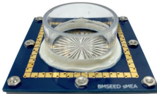
Figure 4. A commercial stretchable MEA on a PDMS substrate manufactured by BMSEED. The PDMS substrate is the transparent rubbery area visible within the cell culture ring in the figure. (BMSEED, 2021)
