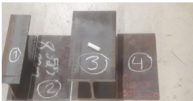
Figure 3 Steel sections and plates from which the test coupons were cut for material testing.
