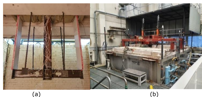
Figure 2 Test furnace arrangements including (a) a photographic image of the specimen inside the furnace before testing and (b) the loading jacks outside of the furnace
