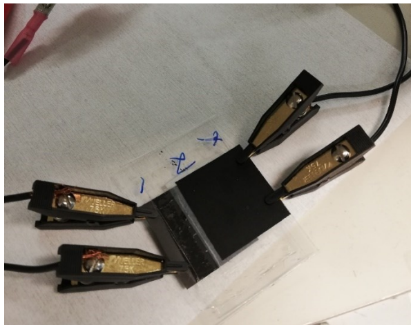
Figure 30. Laminated face to face supercapacitor connected to Maccor 4300 test system using crocodile clips during the measurement process
