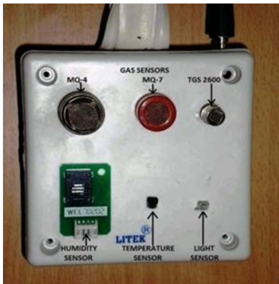
Figure 4. Wireless sensor node:(a) External appearance , (b) the detailed node architecture [6]
