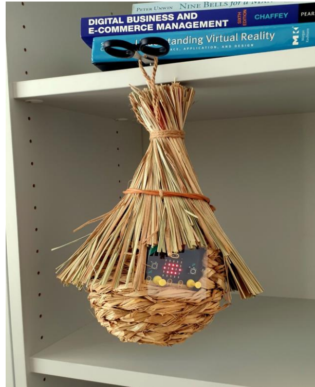
Figure 1: Temperature sensor “Sauron”, a MicroBit-based interactive artefact.
