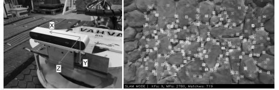
Fig. 2. The left image shows the stereo camera attached to the gripper. The camera's coordinate system is also shown. The right image displays an example view of the detected ORB features during SLAM.
