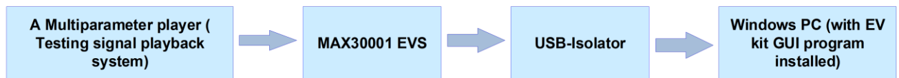
Figure 21 Diagram showing the connected devices and the data flow direction during each test.
