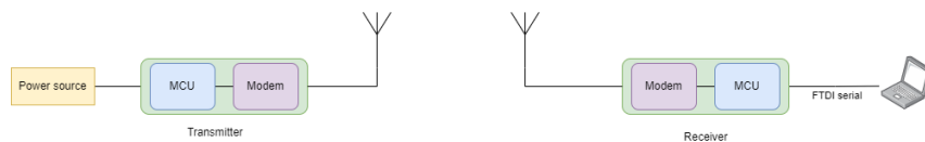
Figure 5.1. DECT-2020 test setup for measurements.
