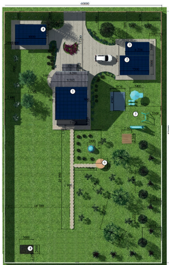
fig. 2. Plan of a private residential plot: 1-residential house, 2-garage, 3-greenhouse, 4-utility-building, 5-playground, 6-gazebo, 7-compost pit for organic waste
