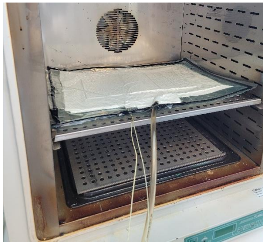
Figure 21: Vacuum bag inside the oven with thermocouples and vacuum ready for curing process
