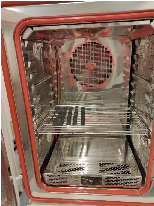
Figure 24: SLS Grease ETW samples inside the environmental chamber
