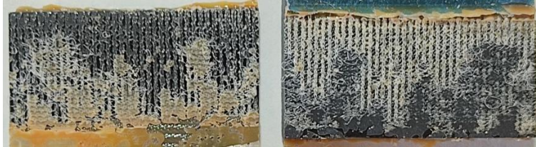
Figure C 1: Representative images of contaminated and non-contaminated DSJ failure surfaces for each surface treatment
