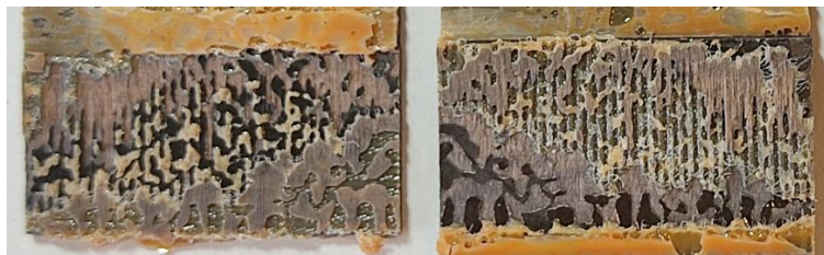
Figure 35: Representative failure surfaces of each surface treatment applied to DSJ samples
