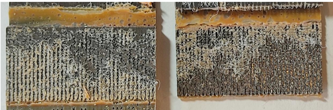
b) Cohesive failure (DSJ Jet fuel, sample 5, F&E interface)
