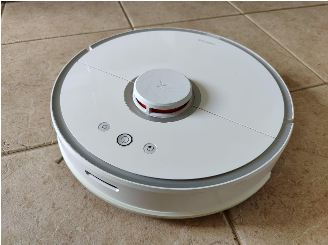
Figure 3. Image of a Roborock S5 which has laser distance sensor mounted on top of the unit.
