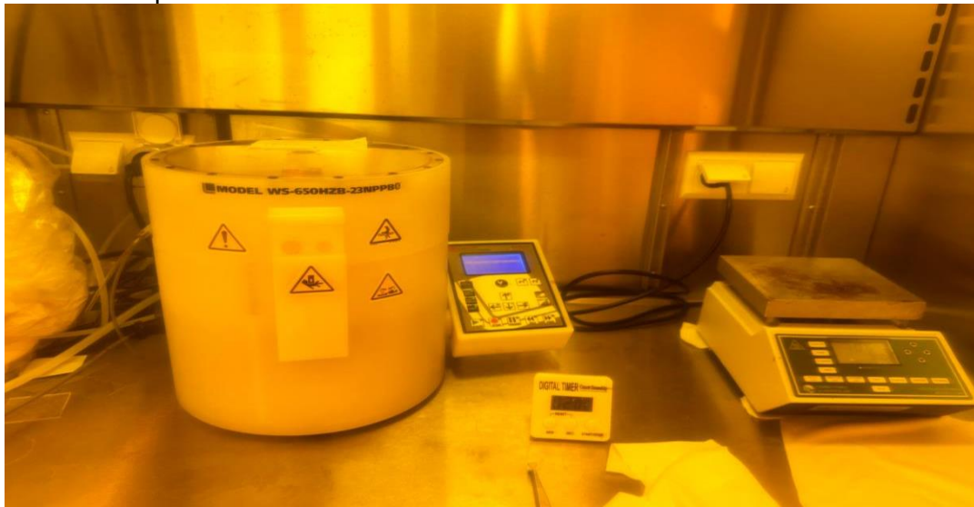
Figure 18: SU-8 coating in the clean room.
