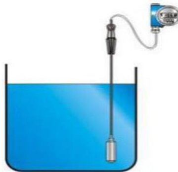
Figure 1: Liquid level measurement with sensor, image taken from Renkeer blog portal [32].
