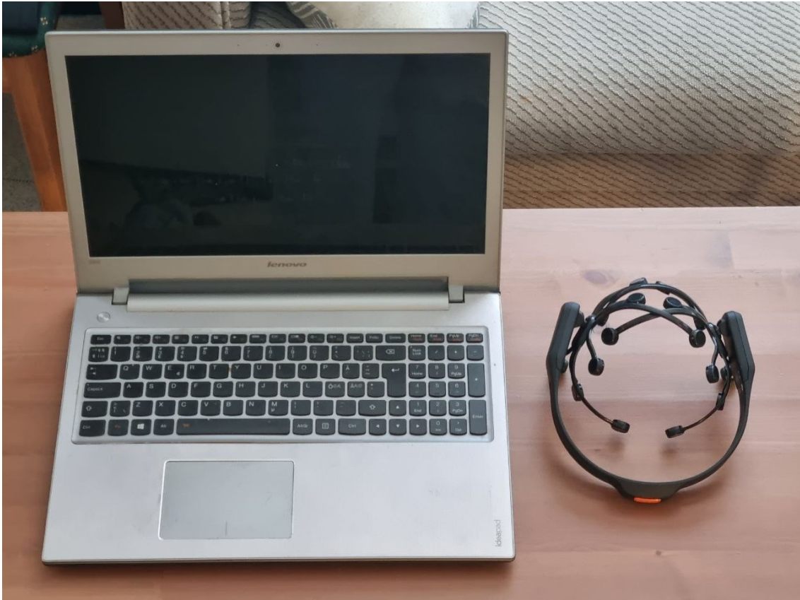
Image 2: The experimental test hardware setup: Lenovo Z500 laptop computer, and the Emotiv EPOC BCI headset.
