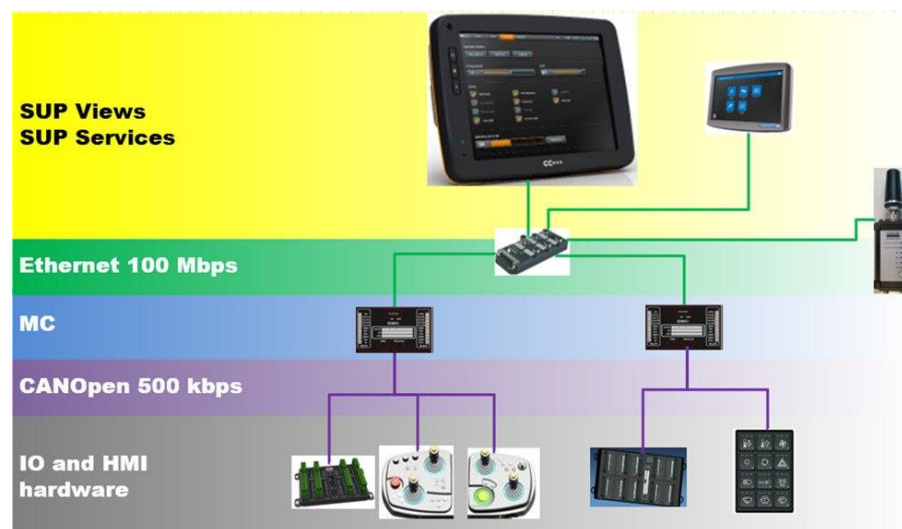
Figure 3. Architecture layers and hardware [6, p. 7].
