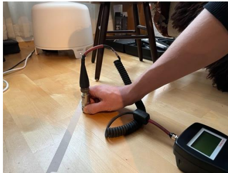
Figure 10. Measuring with a vibration meter from the floor the vibrations that subwoofer produced at a 60 Hz test tone.
