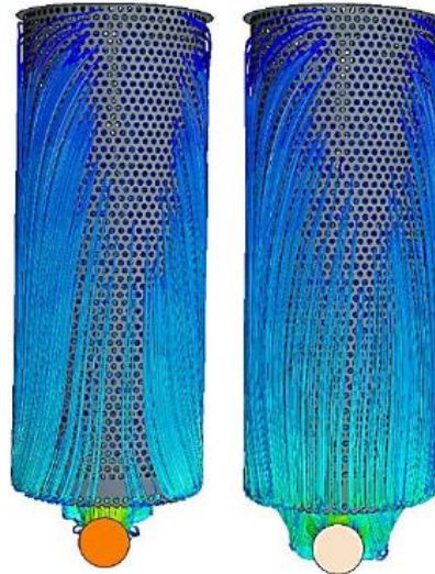
Figure 9: Velocity magnitude of streamlines around the perforated support tube [18]
