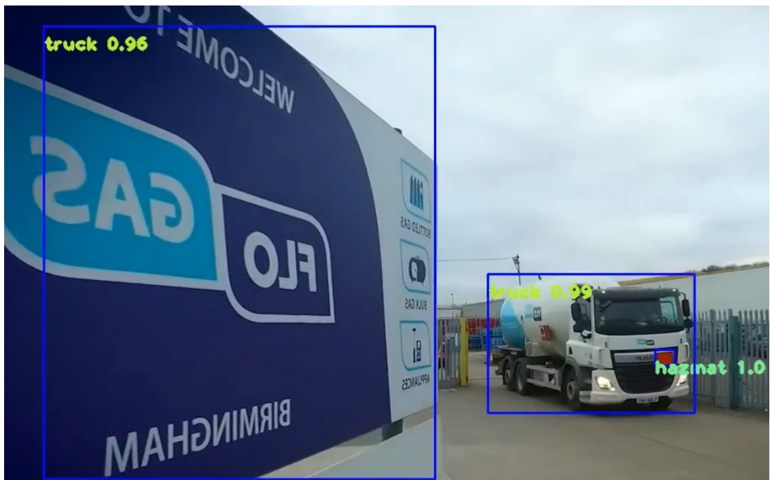
Figure 6.8. Visual inspection of the model's detections can highlight the types of false positives and negatives that the model has difficulty with, which can guide additional data collection. In this example, YOLOv4 416x416 produced a false positive detection of a truck with high confidence, in addition to correct detections..
