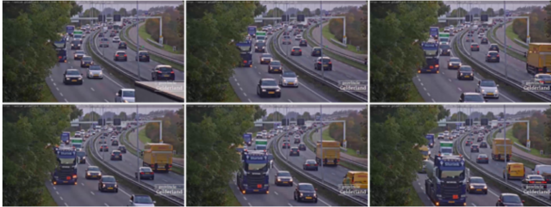
Figure 4.2. Access to live video streams allows the capturing of the same object over multiple frames, which can significantly increase the speed of data collection. In the image, the same truck carrying dangerous goods is captured over multiple frames.
