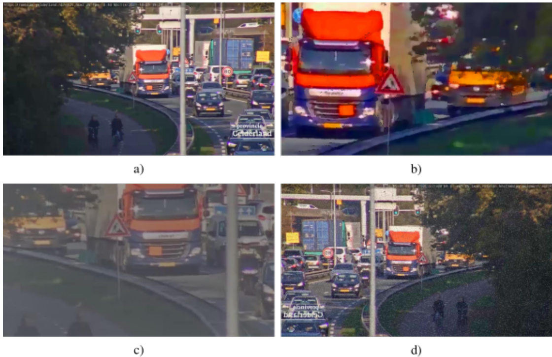
Figure 4.3. Examples of data augmentation in the dataset: a) original image, b) blur (cartoon) + horizontal flip + zoom in, c) reduced contrast + zoom in and d) salt & pepper noise + horizontal flip.
