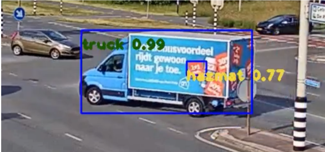
Figure 6.9. The Faster RCNN model incorrectly identified an advertisement on the side of a truck as a hazmat plate. Objects that are shaped like orange rectangles, similar to hazmat plates, can easily lead to false detections.
