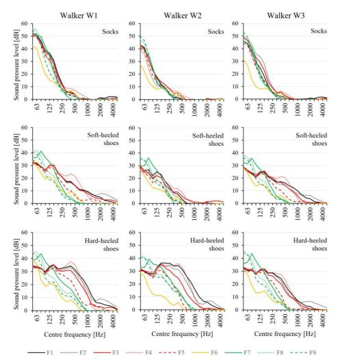
Figure 1: Energetic averages of walking sound spectra based on momentary maxima of  $L_{A,F}(t)$  at 1/3-octave bands in the frequency range 50 to 5000 Hz [9].
