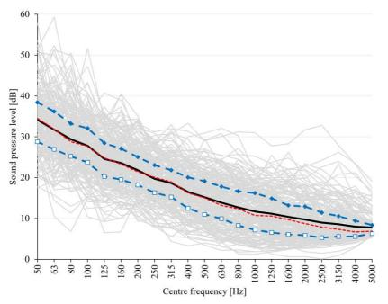
Figure 2: Background noise levels generated by HVAC systems in Finnish dwellings at 1/3-octave bands (grey lines). Continuous black line depicts the mean value. Upper and lower quartile have been shown with dashed blue lines and marked with blue diamonds and white rectangles, respectively; median value of the results has been illustrated with dashed red line. [16, 17]
