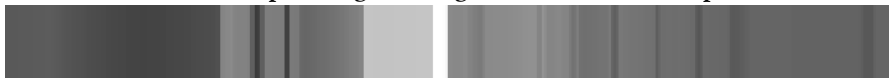
Figure 4.3 © 2021 IEEE. Publication III, Figure 3. Example from the COsy Localization Database (COLD) [58]. The dataset is fully indoors. The greyscale image below is the expanded SICK laser scan spanning 360-degree around the robot (white encodes distances at and above 8 m and black is 0 m). The completely white strip in the middle of the scan is the narrow view into the room on the other side of the corridor that measures 8 meters or more from the sensor. The wider light grey strip on the left side of the white strip is the corridor wall. The rest of the readings are from inside the room and thus closer by.
