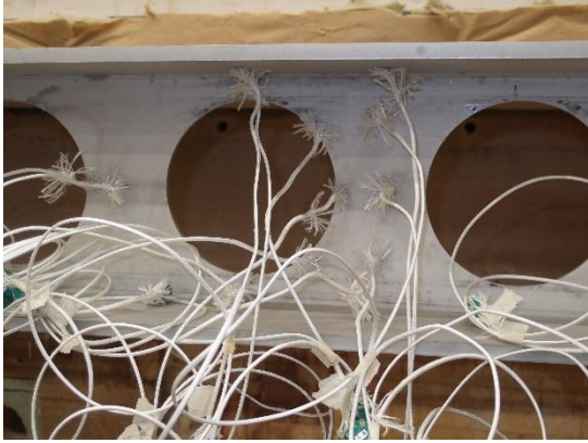
Fig. 5. Locations of the thermocouples in the beam at the mid-span.
