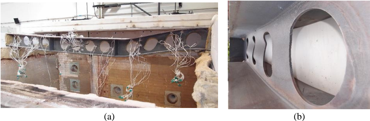
Fig. 8 Images from the test specimen after testing including views of (a) the full member and (b) web-post buckling.
