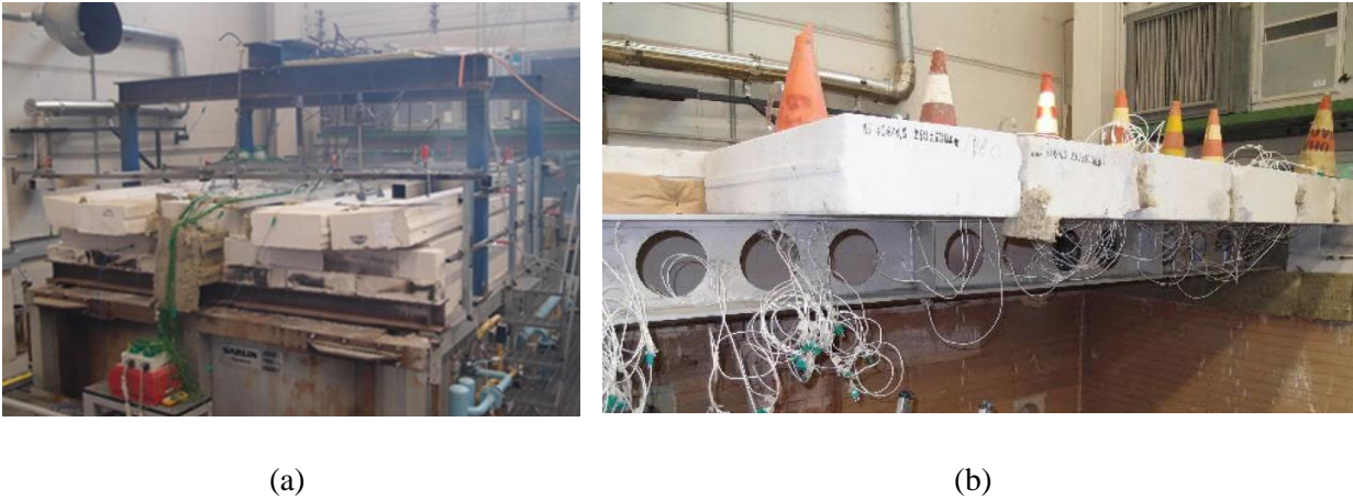
Fig. 4 Images from the test including (a) the loading arrangement above the furnace, and (b) the specimen before testing, including the concrete blocks on the top flange.
