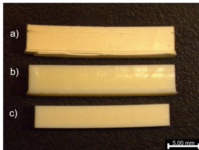
Figure 50: Microscopy image of recipes 5 (75 vol-% DDDA, 5 vol-% PEGMA200, 20 vol-% PEG) (a), 7 (40 vol-% DDDA, 40 vol-% PGTA, 20 vol-% PEG) (b) and 8 (25 vol-% DDDA, 25 vol-% PGTA, 30 vol-% ECC, 20 vol-% PEG) (c) samples after 24h scCO 2 extraction.
