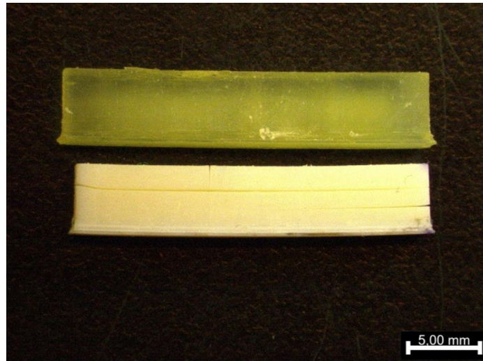
Figure 45: Microscopy images of recipe 6 (37.5 vol-% DDDA, 5 vol-% PEGMA200, 37.5 vol-% PGTA, 20 vol-% PEG) after 24 h scCO 2 exposure in 80 bars (up) and 100 bars (down) at 40 °C.
