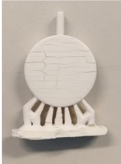
Figure 43: Lithoz Lithalox HP500 green body sample after 1.5h in 100bar and 40°C in scCO 2 .
