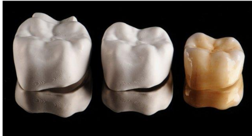
Figure 16: SLA-printed zirconia tooth crown restoration after printing (left), debinding (middle), sintering and coloring (right) [85].
