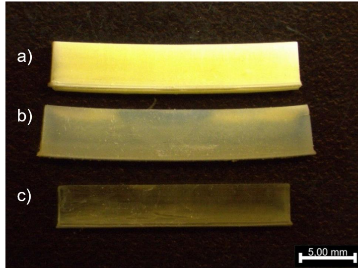
Figure 69: Microscopy images of recipe 8 (25 vol-% DDDA, 25 vol-% PGTA, 30 vol-% ECC, 20 vol-% PEG) after 2h scCO_2 without solvent (a), 2h with EasyClean (b) and 2h with ethanol as co-solvent (c).
