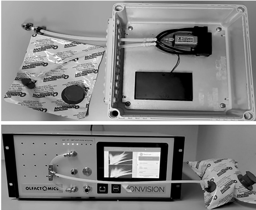
Figure 1. Above: the pump used to aspirate nasal air. A collection bag at the end of Teflon tube and a nasal olive at the end of another Teflon tube. Below: the DMS device attached to the full collection bag and ready for a measurement.
