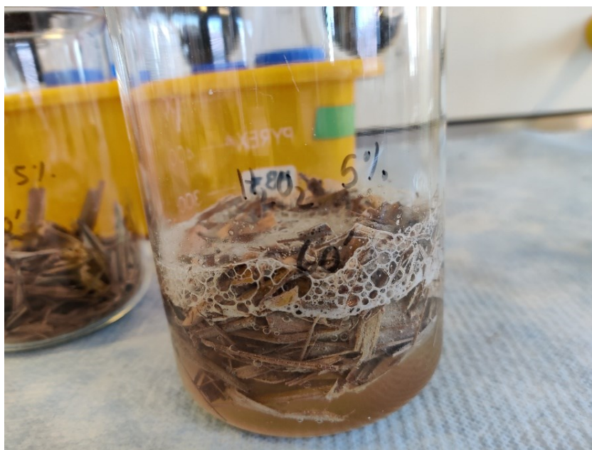
Figure 8. 5% H_2O_2 reaction with molded residues
