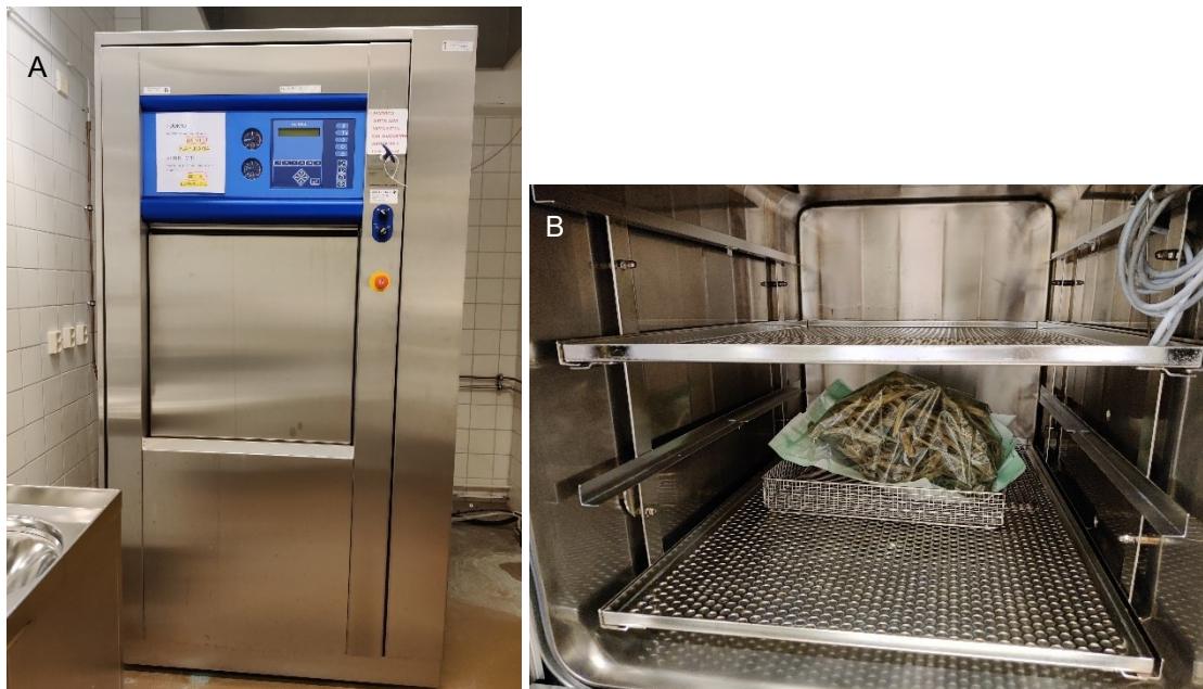
Figure 12. (A) Getinge HS Lab Steam Sterilizer, and (B) the sample bag placed inside the sterilizer
