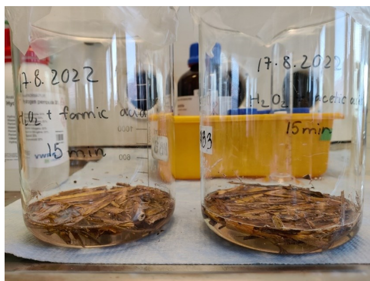
Figure 9. Acid/H 2 O 2 reactions with molded samples
