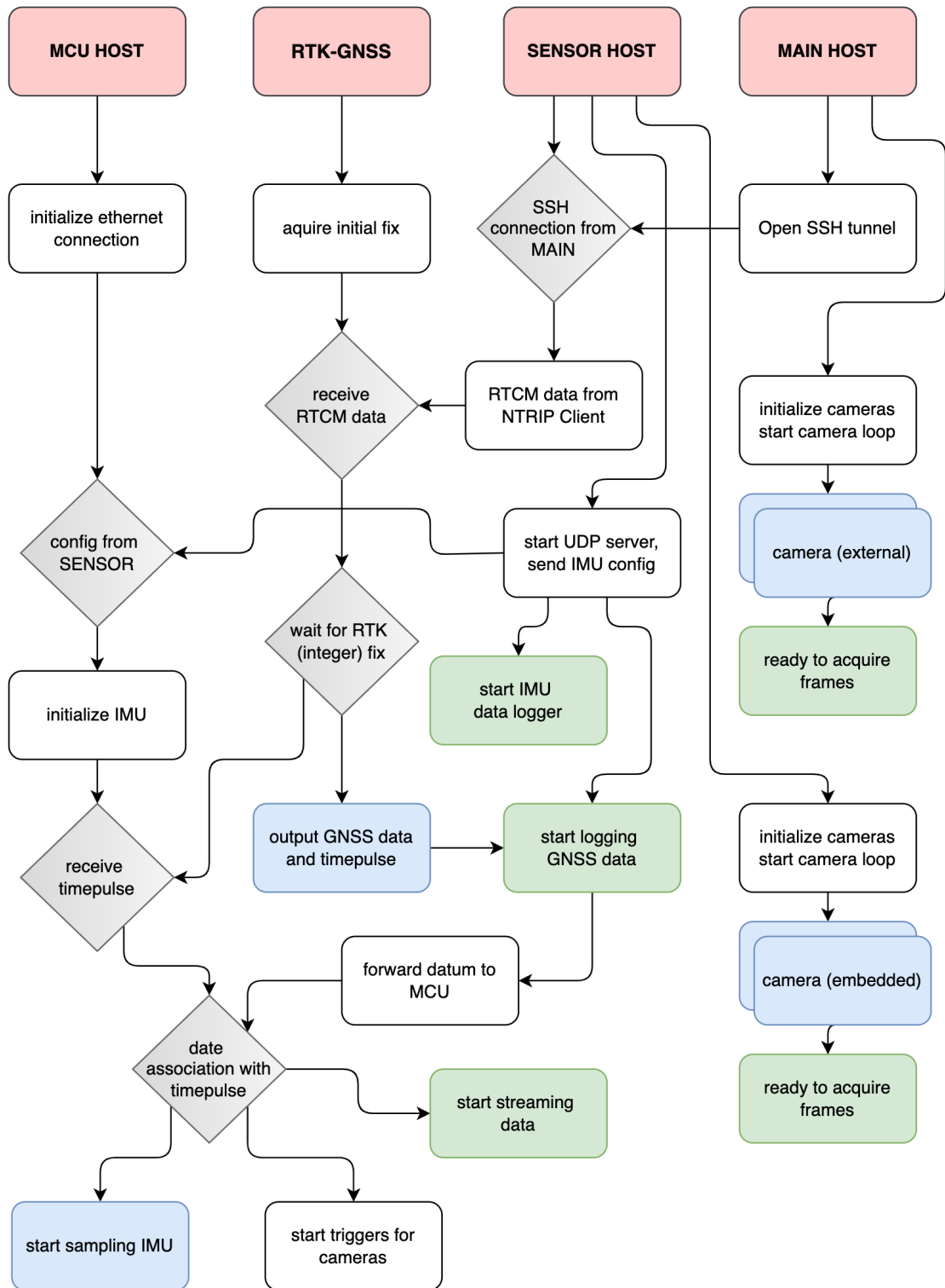
Figure 4.3. Startup sequence and temporal synchronization, the subsystems are presented on the top row, green blocks represent finished startup for software components and blue ones for hardware sensors. Grey diamonds are non-bypass decision points when subsystem has to wait for another subsystem to provide a service.
