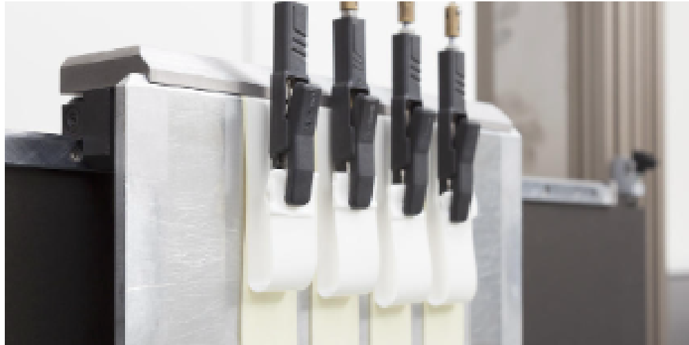
Figure 22. Test assembly for measuring low speed release force [56, p. 12]
