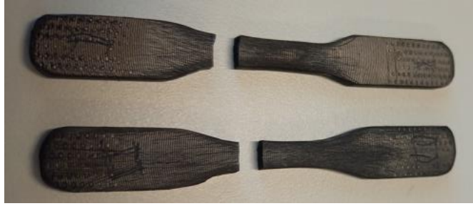
Figure 25. Tensile test specimens of Vespel after the testing.
