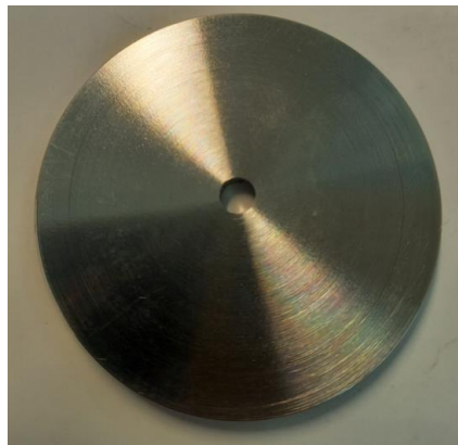
Figure 63. Worn disk after testing with Tivar.
