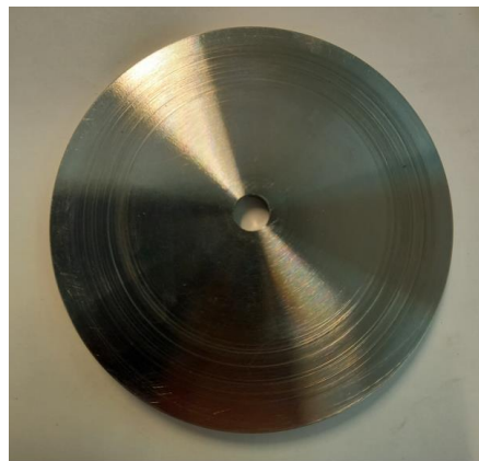
Figure 61. Worn disk after testing with UTEC6540.
