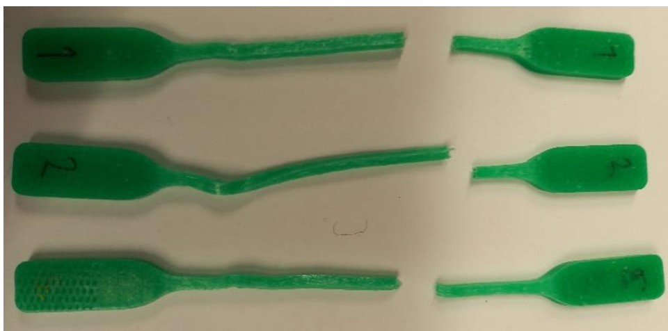
Figure 24. Tensile test specimens Tivar after the testing.
