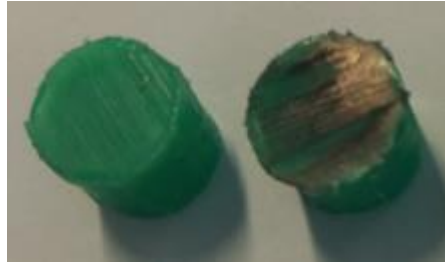
Figure 58. Worn samples of PE1000R.
