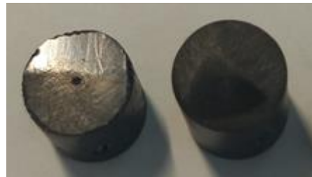
Figure 60. Worn samples of Vespel.
