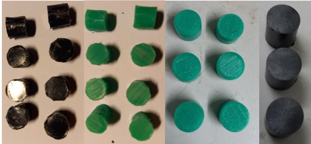
Figure 11. Pin-on-Disk samples of UTEC6540, PE1000R, Tivar and Vespel, from left to right.
