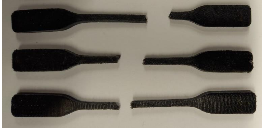
Figure 22. Tensile test specimens of UTEC6540 after the testing.
