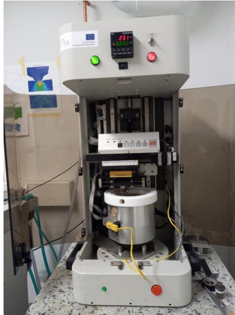
Figure 10. CETR UMT-2 Pin/Ball-on-disk equipment.
