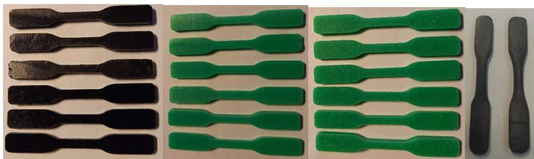
Figure 7. The tensile test specimens of UTEC6540, PE1000R, Tivar and Vespel, from left to right.
