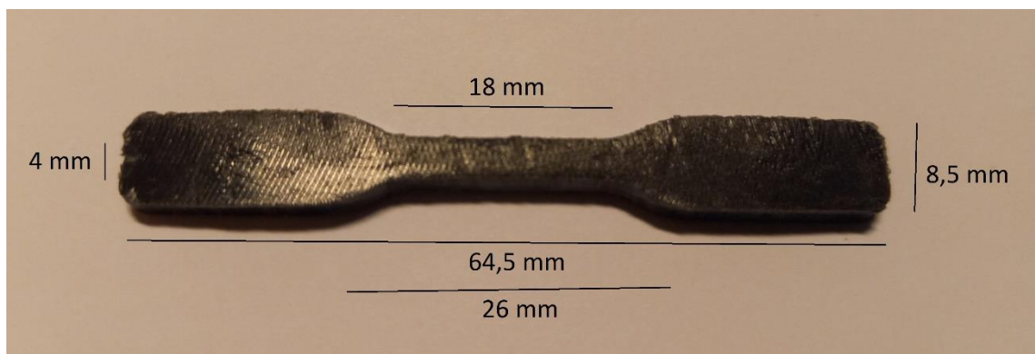
Figure 6. Dimensions of the tensile test specimens.
