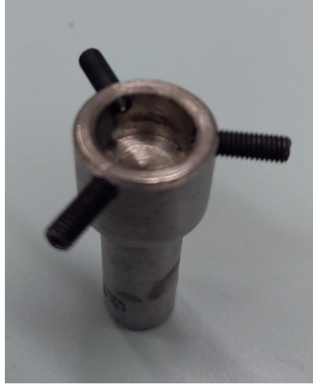
Figure 13. Sample holder with a sample cavity diameter of 10 mm.
