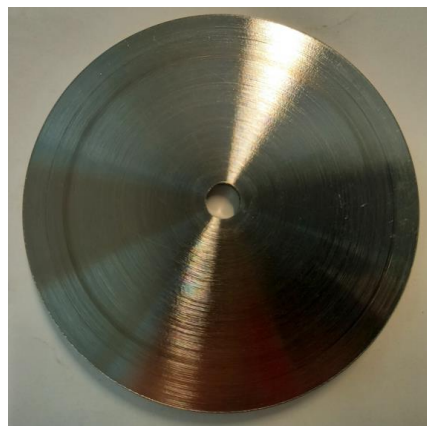
Figure 64. Worn disk after testing with Vespel.
