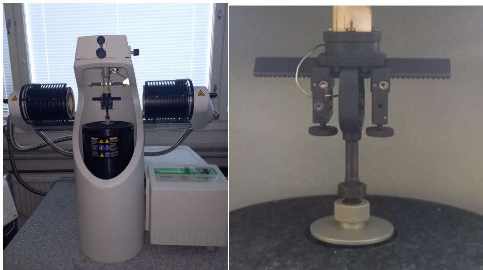
Figure 8. Dynamic Mechanical Analyser (DMA) DMA/SDTA861 (Mettler Toledo) with three-point bending set-up.
