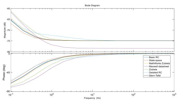
*Figure 57.* Bode-plot when excitation signal amplitude is 1 A and initial voltage 2.13 V
