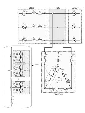
Figure 4. Delta connected full-bridge MMC STATCOM [12]
