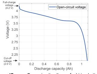
Figure 17. Open circuit voltage of a Li-ion battery [33]
