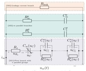
*Figure 45.* Simplified series model of a supercapacitor cell [64]
