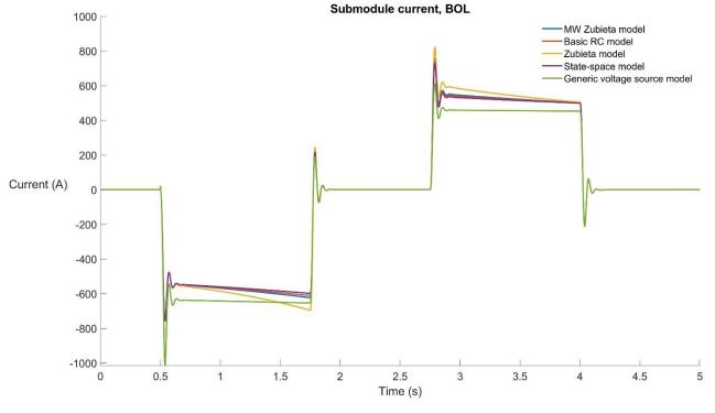
*Figure 65.* Submodule current with one battery and four supercapacitor models
