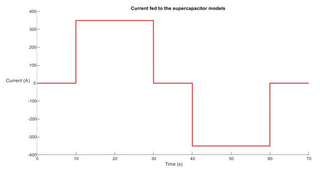
*Figure 51.* Injected supercapacitor current
