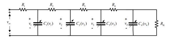
*Figure 39. Transmission line model of a supercapacitor* [94]
