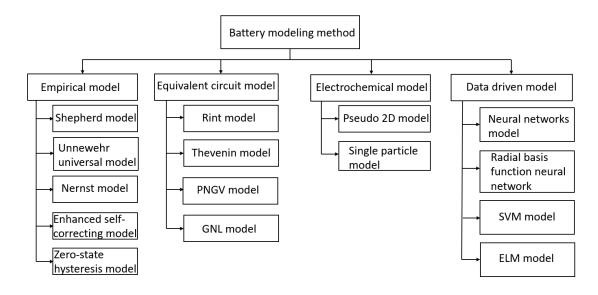
Figure 30. Battery modelling methods, modified from [86]
