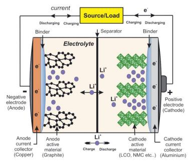
Figure 14. Li-ion battery while charging/discharging [33]
