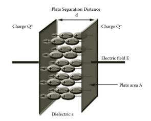
*Figure 12.* Charged parallel plate capacitor [22]
