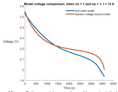
Figure 38. Battery model comparison with constant discharge current
