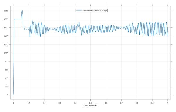
Figure 68. Supercapacitor voltage in a submodule
