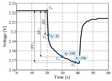
*Figure 35.* Voltage response of the battery to a discharge current pulse [92]
