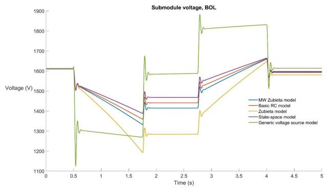
*Figure 64.* Submodule voltage simulation results with one battery and four supercapacitor models
