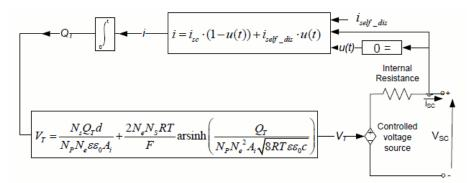
*Figure 49.* Simulink supercapacitor model based on controllable voltage source [105]
