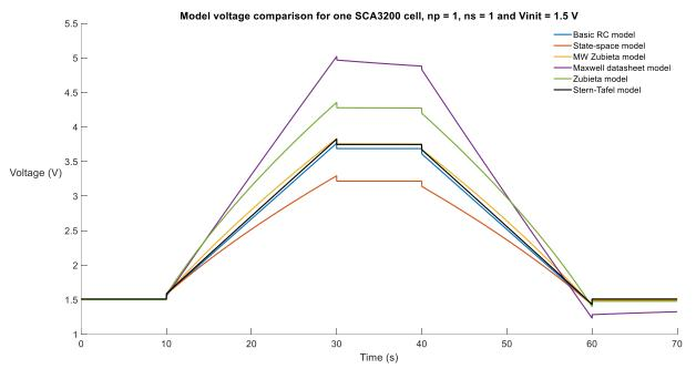
Figure 53. Supercapacitor simulations with initial voltage of 1.5 V
