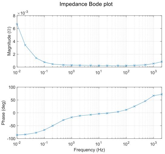
Figure D: 3 V, 3000 F Supercapacitor impedance. Initial voltage 0.7 V
