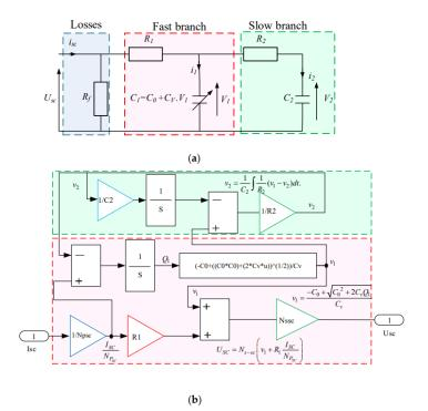
*Figure 47.* Faranda equivalent circuit a) and Simulink model b) [102]
