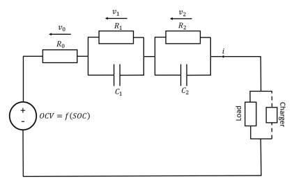
*Figure 33.* General Li-ion circuit diagram
