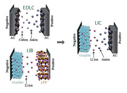
*Figure 29.* LIC structure combining properties from EDLC and LIB [78]
