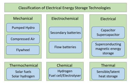
Figure 13.Energy storage classification based on the form of stored energy[26]
