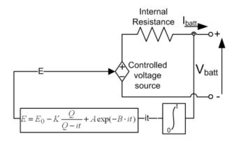
*Figure 31.* Non-linear voltage source battery model [88]
