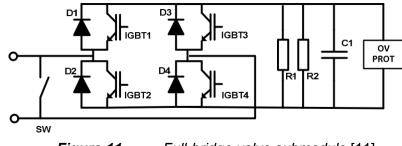
Figure 11. Full-bridge valve submodule [11]
