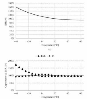
*Figure 28.* Temperature dependency of supercapacitor equivalent series resistance and capacitance [58]
