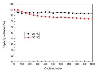
*Figure 18.* LTO cell capacity retention at 3 C current at different temperatures [56]
