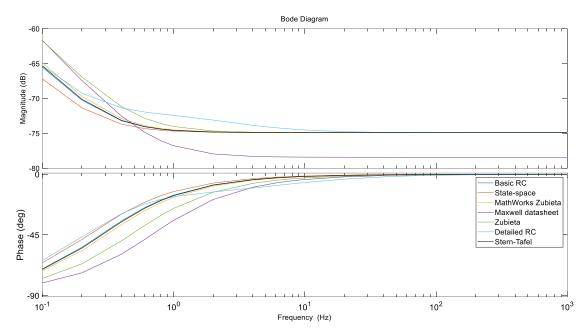
*Figure 58.* Bode-plot when excitation signal amplitude is 350 A and initial voltage 2.13 V
