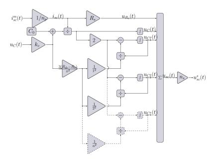
Figure 46. Nonlinear supercapacitor bank block diagram [64]
