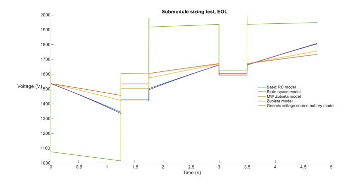
*Figure 63.* Constant power test for energy storage models with EOL conditions
