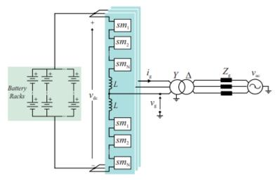
*Figure 8.* Centralized energy storage topology. Possible for DSCC, DSBC and DSHC topologies [14]
