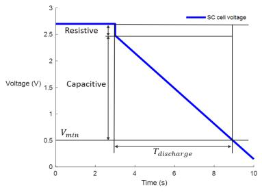
*Figure 24.* General discharge profile of a supercapacitor at constant current
