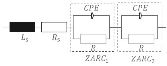
Figure 34. Electrical equivalent circuit based on ZARC elements [91]
