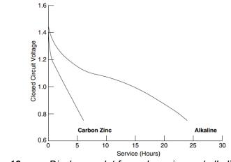
*Figure 16.* Discharge plot for carbon-zinc and alkaline batteries [48]
