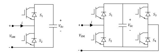
Figure 6. Half-bridge and full-bridge submodule topology
