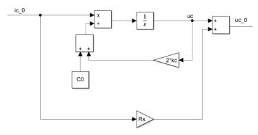
Figure 43. Large signal supercapacitor block diagram
