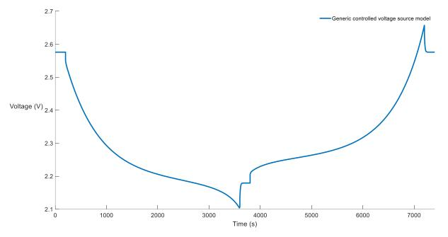
Figure 32. Generic voltage source model simulation result for a battery cell
