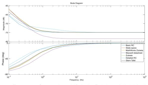
*Figure 55.* Supercapacitor model Bode-plots. Excitation amplitude 350 A and initial voltage 0 V
