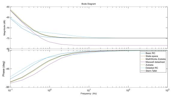
*Figure 56.* Bode-plot when excitation signal amplitude is 1 A and initial voltage is 0 V
