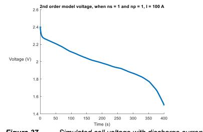
Figure 37. Simulated cell voltage with discharge current of 100 A
