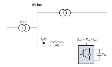
Figure 9. Simplified single-line diagram of a STATCOM
