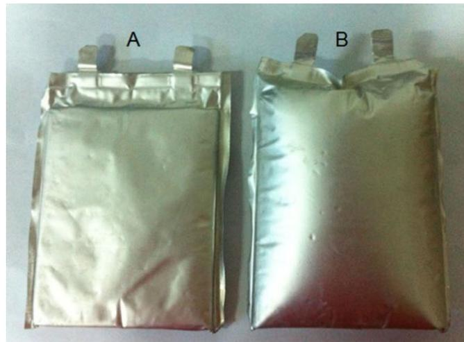
**Figure 19.** LTO cell gas build-up with 3 C current at A) 25°C and B) 55°C after 1000 cycles [56]
