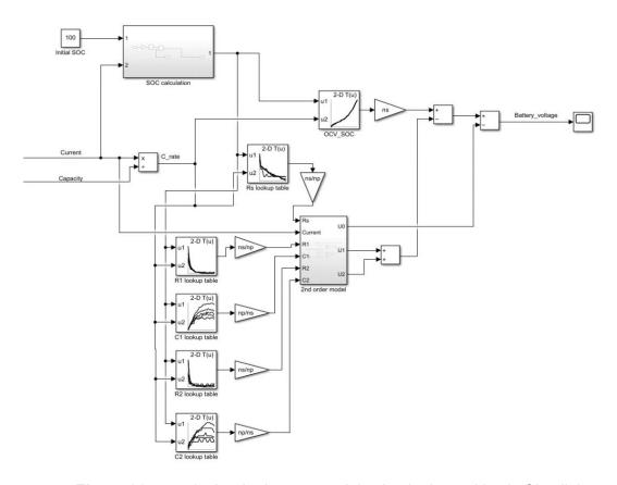
*Figure 36.* 2nd order battery model using lookup-tables in Simulink
