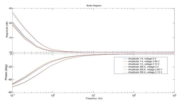
Figure 59.MathWorks Zubieta model Bode-plot with different excitation signal<br/>amplitudes and initial supercapacitor voltages
