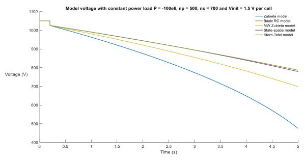
Figure 54. Constant power discharge simulation
