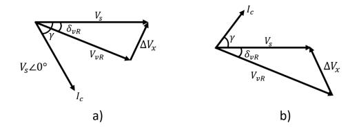
*Figure 10.* Leading a) and lagging b) space vector representations of STAT-COM
