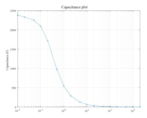
Figure C: Frequency dependent supercapacitor capacitance for a 3 V, 3000 F cell. Initial voltage 0.7 V
