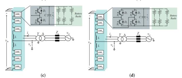
*Figure 7.* STATCOM topologies for distributed energy storage integration: a) SSBC, b) SDBC, c) DSCC and d) DSBC [14]
