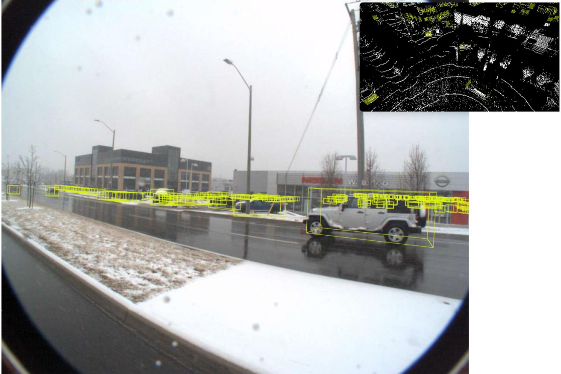
Figure 5. Image and LiDAR scene from CADCD. The image shows multiple bounding boxes in the nearby building’s wall. This is because the annotation data does not mention object visibility in camera images. Adapted from [28].
