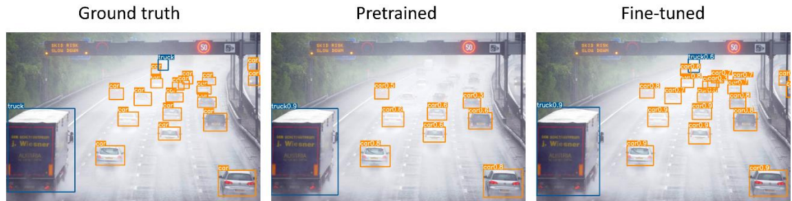
Figure 23. Ground truth, pretrained and 50-image fine-tuned detections on DAWN dataset's rain category.
