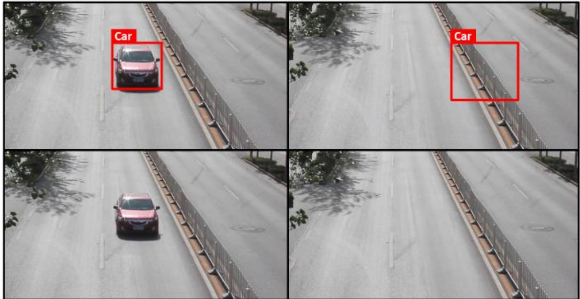
Figure 11. The upper left image depicts a true positive detection and the upper right images a false positive one. The lower left image shows a false negative as the car in the image is not detected. The lower right is completely true negative as there are no objects or detections.
