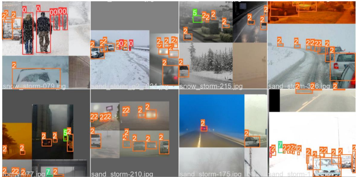
Figure 10. YOLOv5's Mosaic enhanced training images created by mixing randomly scaled and clipped base images.
