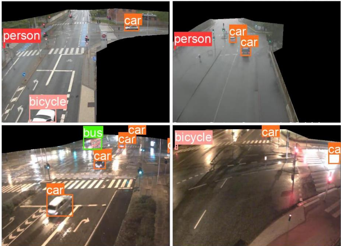
Figure 7. Example images from AAU RainSnow dataset showing variation and challenging detection tasks but also some mistakes. Black areas in the images represent the masks for unlabelled areas.
